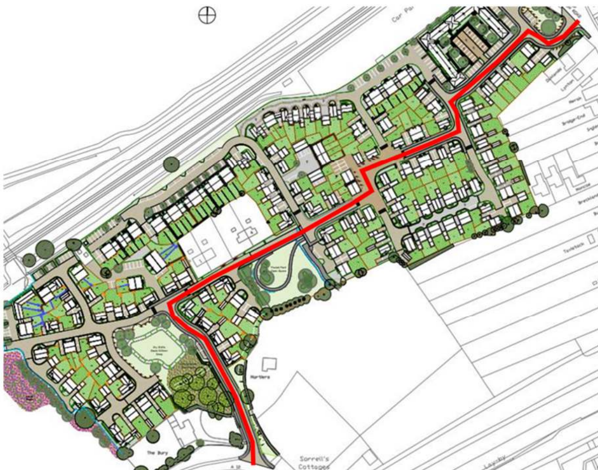
Plate 5.10 Temporary through route
